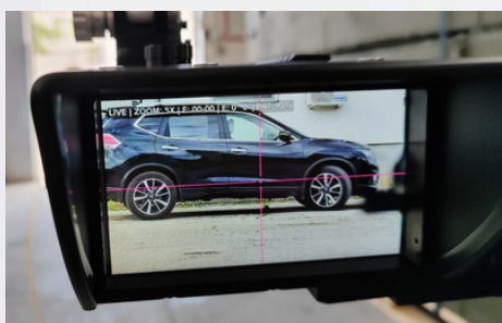
Picture from the PGDN-9VIR during the day at 5x magnification, target distance 100m.
